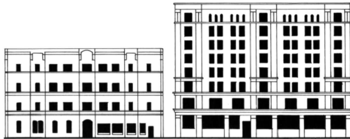
Elevation Showing Relationship of Window to Wall
